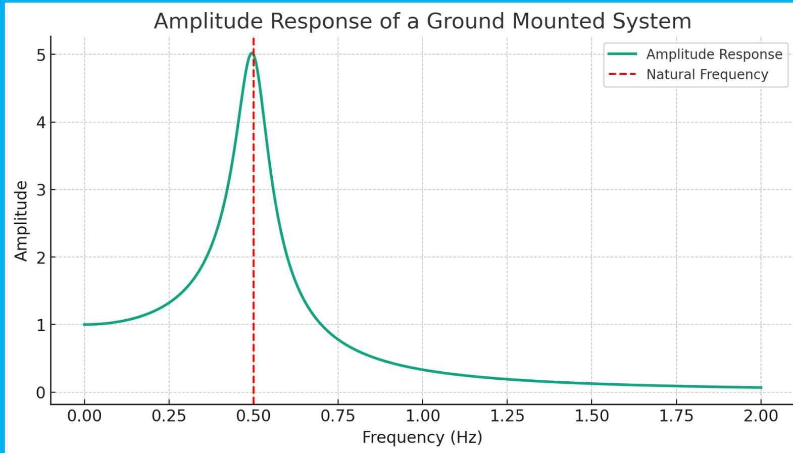
Graph showing the amplitude response of a system across a range of frequencies, highlighting the peak at the natural frequency.
