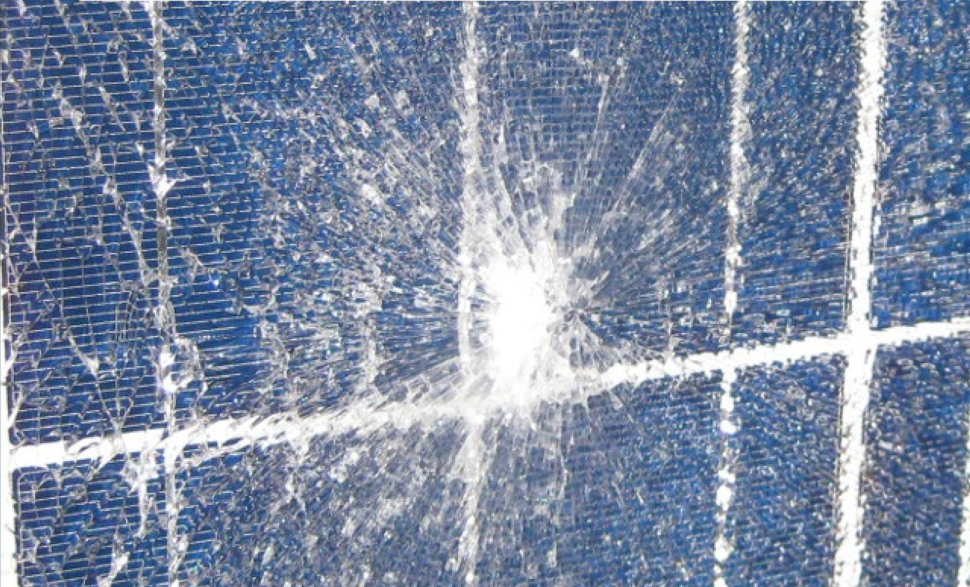
Broken solar panels - lightning damage, shattered glass
